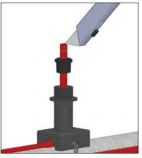
2. Score the outer insulation 1/2 inches from the end of cable. Lightly cut the outer jacket up the center to end of heating cable and remove the jacket from the cable.
