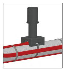
**6.** Tighten end cap until it bottoms out on pipe standoff.
