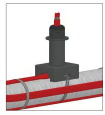
**4.** Adjust cable leaving 1" past the end of the grommet and insert the grommet into the pipe standoff. Attach extra cable to pipe as shown.
