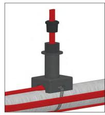
1. Insert cable without the braid through pipe standoff and grommet as shown. Attach pipe standoff to pipe with pipe straps (Trasor model PS not included). Leave braid outside of pipe standoff at grommet. For pipes smaller than 1 1/2" diameter a small pipe adapter (Trasor model SPA not included) is required.
