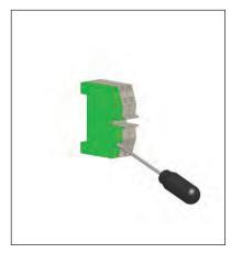
11. Attach 3/4" conduit hub. Use a flathead screwdriver to release the terminal spring clamps and insert cable leads and grounding braid as per wiring diagram on next page. Supply power electrical connections to terminals as shown on wiring diagram on next page. For A T E X a n d I E C E x installations, conduit hub must be an ATEX or IECEx certified component.
