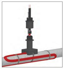
Slide compression fitting over cable. Grommet should be placed inside pipe standoff. Termination boot should be spaced 1/2" from sealing grommet.
