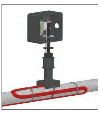
10. Assemble junction box to compression fitting as shown. Tighten locknut until the junction box bottoms out against the lip of the compression fitting.
