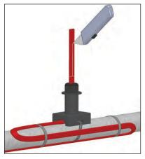
Score the outer insulation 7 inches from the end of the cable. Lightly cut the outer jacket up the center to the end of heating cable and remove the outer jacket from the cable.
