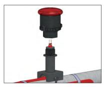
Attach LED Assembly to pipe stand off as shown. Liberally apply RTV over the exposed matrix and leads.
