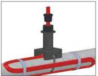
1. Insert heating cable through pipe standoff and grommet as shown. 1-1/2 inches of cable past the should extend grommet. Strap pipe standoff to the pipe with pipe strap (Trasor PS-3 pipe strap is included. Order different sized straps separately, UESL to be mounted vertically only). Then attach extra cable to pipe as shown to create a service loop. For Pipes smaller than 1-1/2 inches diameter a small pipe adapter is required.
