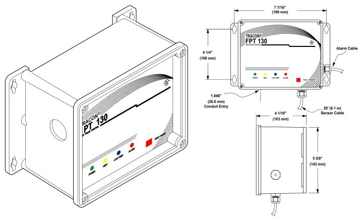
The FPT 130 Heat—Trace Control is a single—point microprocessor—based heat—trace control thermostat. It is ideal for applications which require Ground—Fault Equipment Protection (GFEP). Ideal uses include freeze protection, and other temperature monitoring and control applications.
